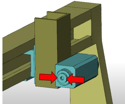
Spindle Diameter Measurement (SDM) = \_\_\_\_\_
