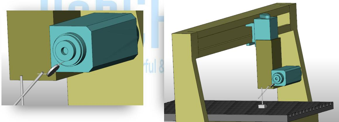
The  $Z_2$  value is the reading from the machine's control to the location shown and takes your indicator back to zero. The  $Z_3$  value is the adjusted  $Z$  value to let us know where the center of the spindle axis is in this position. To get the  $Z_3$  value just subtract the Spindle Radius from the  $Z_2$  value.
